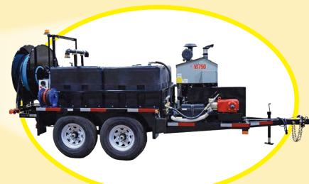
"The whole VJ series is designed specifically for sewer and storm waterline jetting and cleaning," Brown says. "It is ideal for removing blockages, cutting through debris and cleaning out sewer, storm and catch basins. They are perfect as an addition to a larger fleet, or they can stand on their own for smaller jobs."
